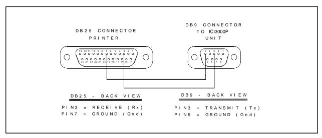
Figure 8. DB25 Printer Connector to DB9 ICI3000P Unit Pin Assignments
